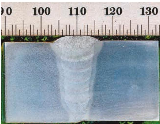
Figure 4. Open root weld.
