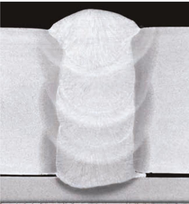
Figure 6. Four passes, square-edge butt weld on 3/4 in. (19 mm) plate.
