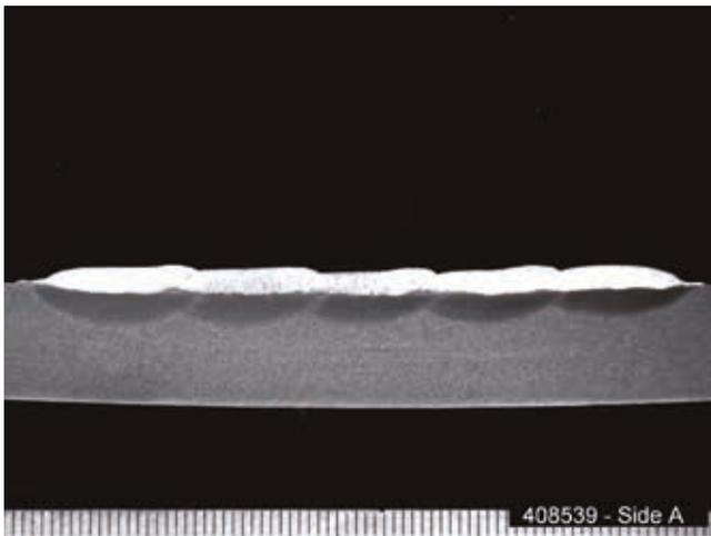
Figure 5. 8.79% Fe with one pass.
