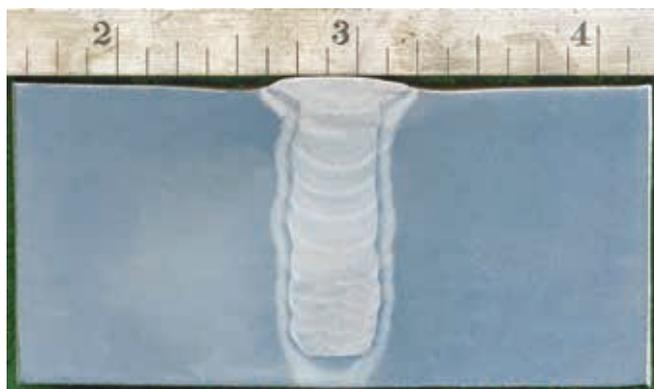
Figure 3. Fill passes on X65 pipe.
